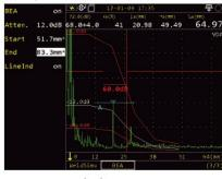
• This function is to help set a gate over an area and adjust the gain for this area regardless of the global gain. It is very useful for inspection of Forgings and Castings with allowing independent gain control of the area under the gate with the BEA for backwall echo monitoring.
