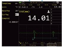
• When there is temperature difference between the calibration block and the detected workpiece, it can be used for temperature compensation. Adjustable range is -10 to 400 °C.
