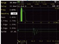
The probe waveform, spectrum and center frequency of the probe can be measured precisely by capturing echoes.
