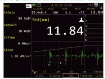
• It can be used for compensating the loss of echo amplitude due to propagation of sound path.
