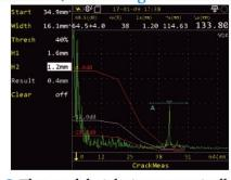
The crack height is automatically calculated with this function.
