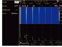
Display A-scan echo in imaging mode based on time or encoder, so as to achieve more intuitive test result for easy observation and analysis.
