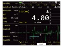
After setting the coating velocity, coat and base material thickness can be displayed at the same time.
