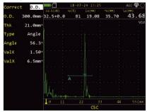
• For depth and horizontal distance correction when testing circumference with an angle probe.
